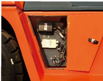
独立集成电控箱 Independent integrated electric cabinet
