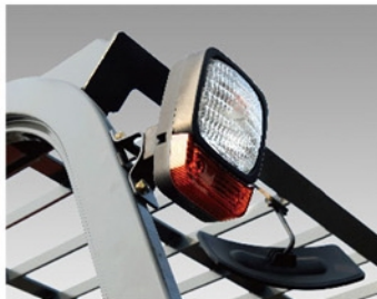
标配LED信号灯 LED signal (standard configuration)
